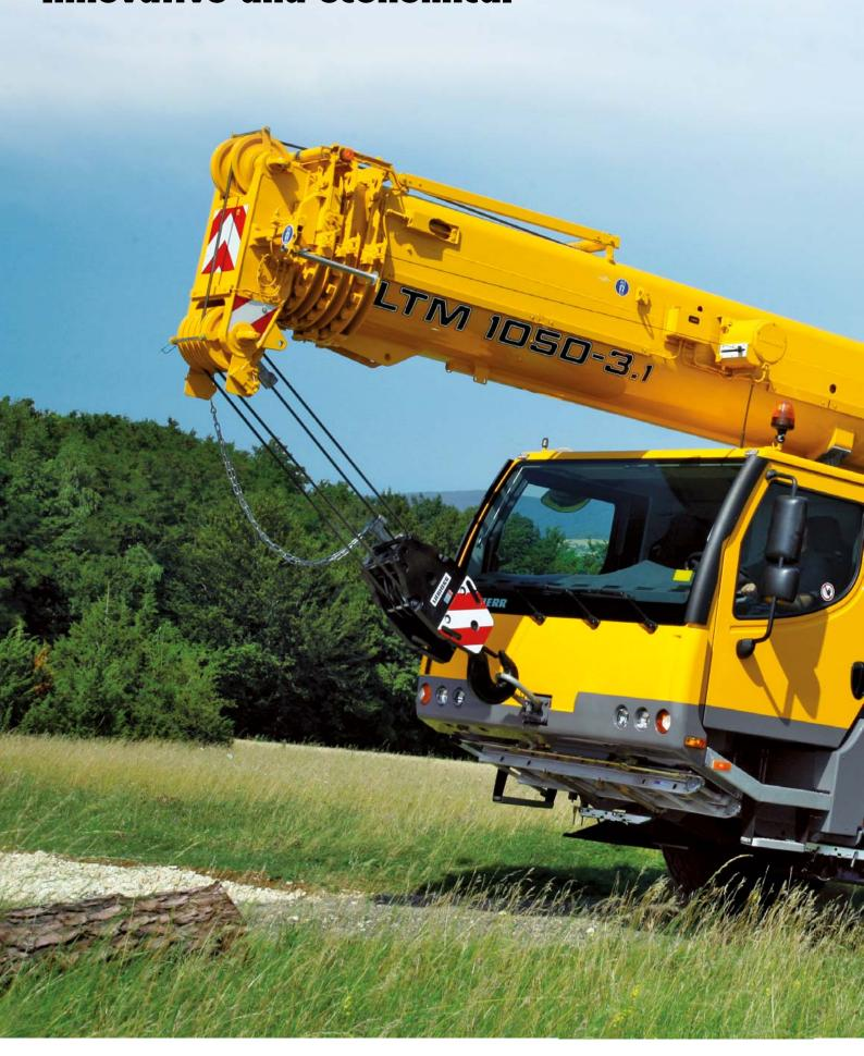
The Liebherr LTM 1050-3.1 mobile crane is characterised by its long telescopic boom, strong lifting capacities, exceptional mobility and comprehensive comfort and safety equipment. This 50-tonne crane features top-of-the-range technology for more effectiveness in practical operation.
